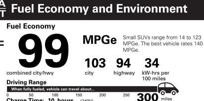
kW-hrs per 100 miles **300** Charge Time: 10 hours (240V) Fuel Economy & Greenhouse Gas Rating (tailpipe only) Smog Rating (tailpipe only) Annual fuel COST \$750
