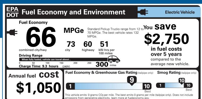
Actual results will vary for many reasons, including driving conditions and how you drive and maintain your vehicle. The average new vehicle gets 28 MPG and costs \$8,000 to fuel over 5 years. Cost estimates are based on 15,000 miles per year at \$.14 per kW-hr. MPGe is miles per gasoline gallon equivalent. Vehicle emissions are a significant cause of climate change and smog.
